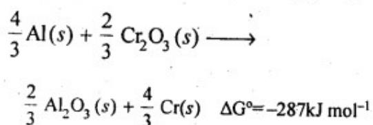
As can be seen  $\Delta_f G^\circ$  is negative, thus, reduction of  $\text{Cr}_2\text{O}_3$  by Al is possible.
